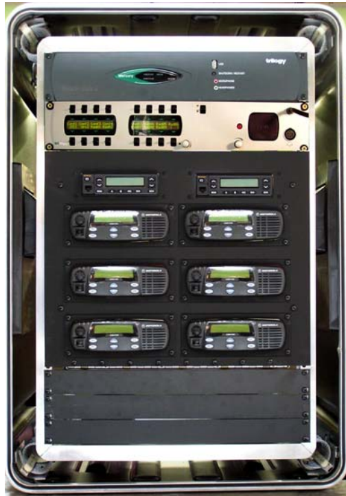
Portable Interoperability Unit Rack mounted with eight radio systems in a shippable shock-mount rugged case
